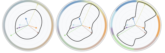
Figure 6. Effect of temperature \tau – With a low value of \tau the representation is easy to optimize as its degrees of freedom have a large support, while if sharp discontinuities are needed, a large value of \tau can be chosen; above \tau = \{1, 5, 25\} .
